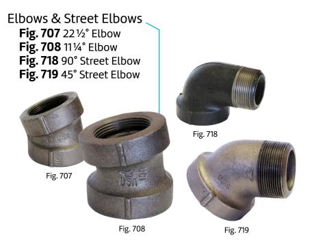
Anvil drainage fittings have sufficient sweep to allow free unobstructed flow. They are made with a shoulder of the same diameter as the inside of the pipe, in accordance with ASME B16.12, Type 1.
